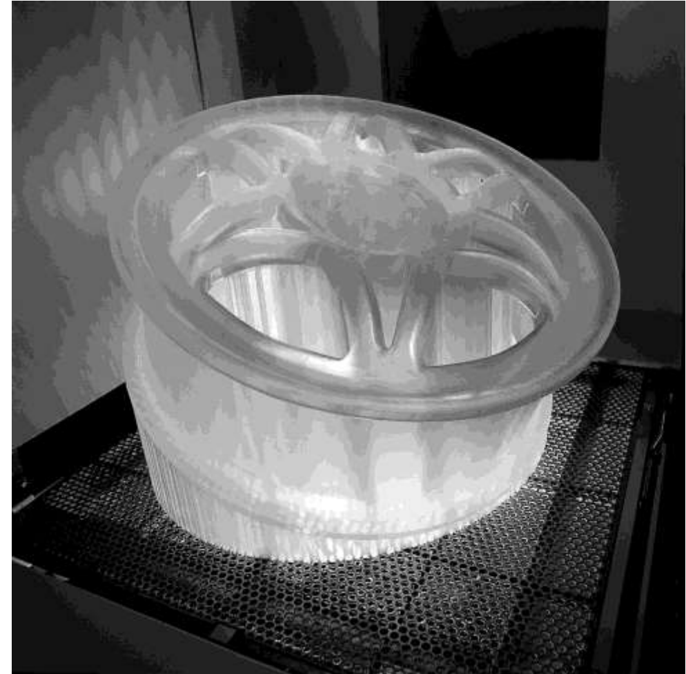
Schematic illustration of the stereolithography process and part of SLA
