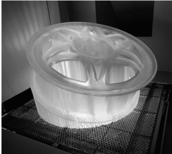
A part produced by stereolithography
