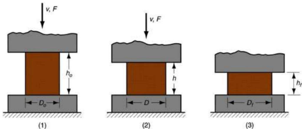
**Figure:** Homogeneous deformation of a cylindrical workpart under ideal conditions in an open-die forging operation: (1) start of process with workpiece at its original length and diameter, (2) partial compression, and (3) final size.
