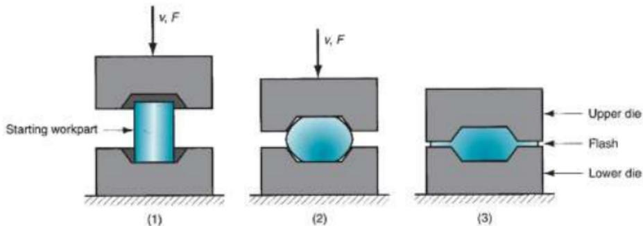
**Figure:** Sequence in impression-die forging: (1) just prior to initial contact with raw workpiece, (2) partial compression, and (3) final die closure, causing flash to form in gap between die plates.
