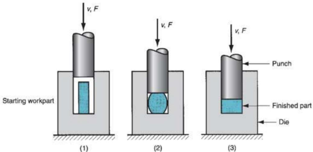
**Figure:** Flashless forging: (1) just before initial contact with workpiece, (2) partial compression, and (3) final punch and die closure
