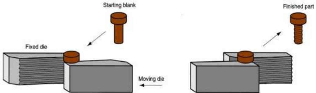
**Figure:** Thread rolling with flat dies: (1) start, and (2) end of cycle.
