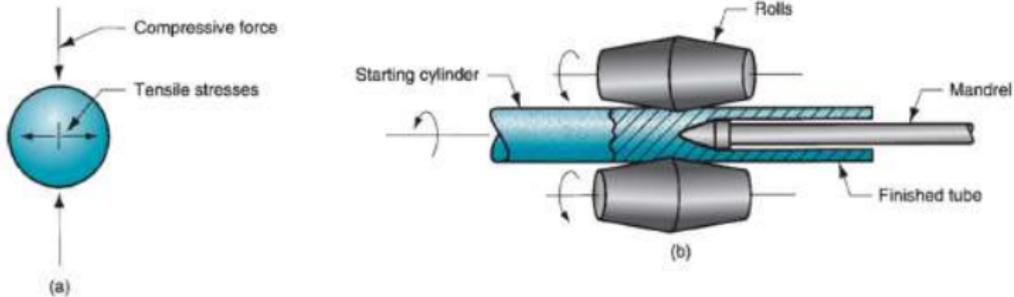
**Figure:** Roll piercing: (a) formation of internal stresses and cavity by compression of cylindrical part; and (b) setup of Mannesmann roll mill for producing seamless tubing.
